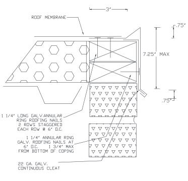
GS SERIES ( GRAVEL-STOP STANDARD ) GRAVEL STOPS ARE AVAILABLE IN VARIOUS METALS. THEY ARE ES-1 TESTED IN 24 GA. STEEL AND .040 ALUMINUM. MAXIMUM TESTED FACE SIZE IS 8". CALL ULTRA SEAM FOR
